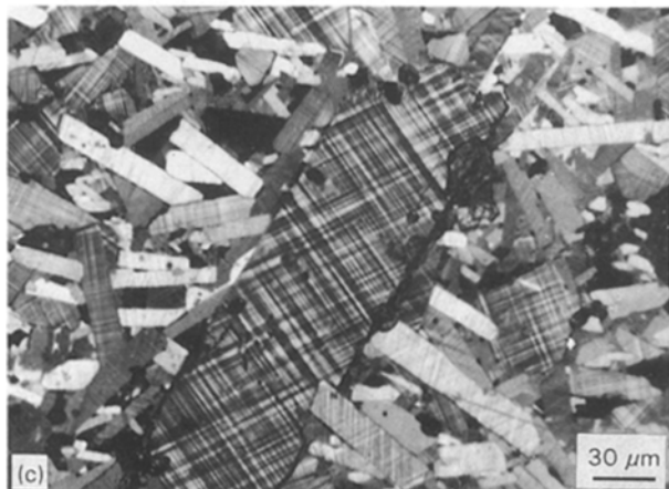
Figure 8 Light polarized optical micrographs of \text{YBa}_{2-y}\text{K}_y\text{Cu}_3\text{O}_{7-x} doped with 2.5 at % \text{K}_2\text{O} : (a) 920 °C, 4 h; (b) 940 °C, 4 h; and (c) 940 °C, 8 h.
